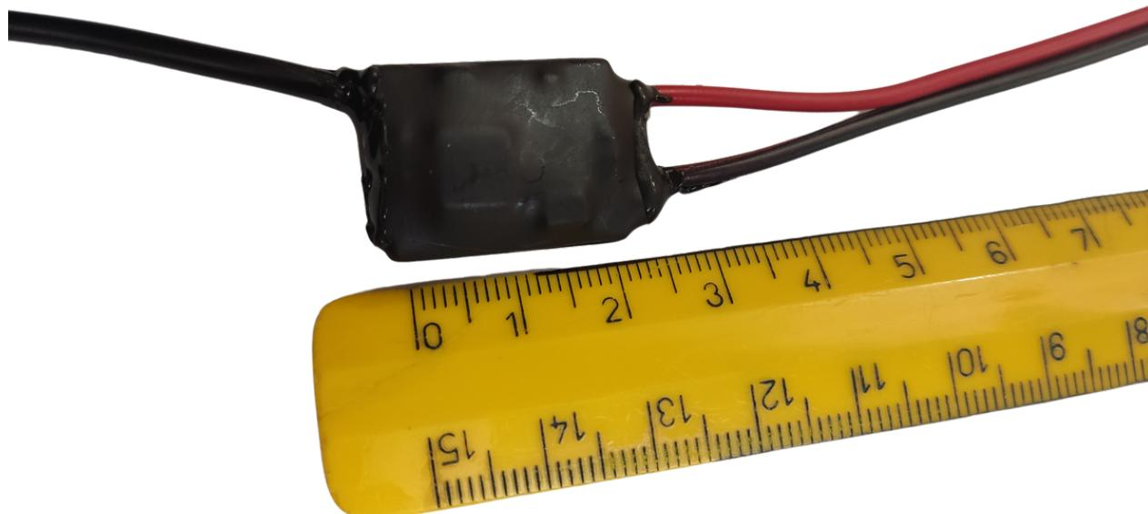
The small dimensions of the micro transformer (just 25 x 17 x 8 mm) allowes it to be easily hidden inside electrical systems in homes or cars to power a GSM bug.
